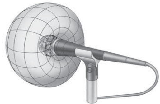
Cardioid (Unidirectional) Microphone
