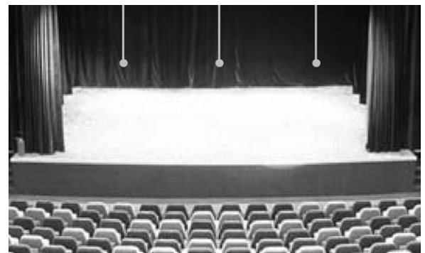
Illustrative example of overhead microphone placement being used to provide area coverage
