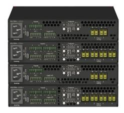
The Voltera® A Series are four half-rack power amplifiers with a total power of 300 or 600 W delivered by two or four channels in a sleek, compact design. The amplifier channels are extremely flexible in that they can individually be selected to drive either 4 ohm, 8 ohm, 70 V or 100 V. They also support power sharing so that up to twice the power can be delivered by any channel. Every A Series amplifier ships with mounting accessories for a variety of mounting options.
